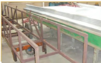
Iron rack without felt protection (unprotected)
